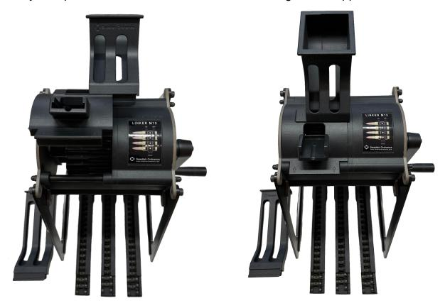
**Step 2:** Load the link magazines. The links only fit in one direction and need to be loaded as in the picture below.
