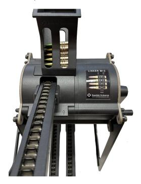
**Step 4:** Crank the handle clockwise. Do not crank anti clockwise. In case of jam, open the lid. When the link magazine is empty fill it or change it for a full one.
