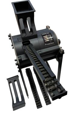
**Step 3:** Insert the link magazine in the linker. The links should slide down as the magazine snaps into place. Fill the hopper with ammunition. The ammunition needs to be pointing in the same direction as in the picture.
